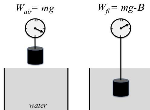
**Figure 1:** Weighing in object in air and in water.
