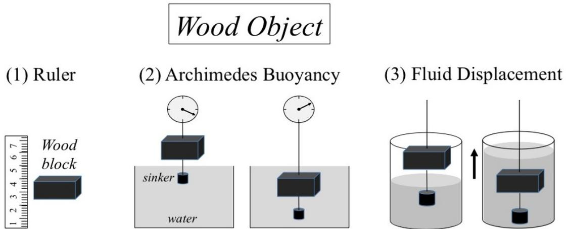
**Fig.3** Three ways of measuring a wood object’s volume  $V$ .
