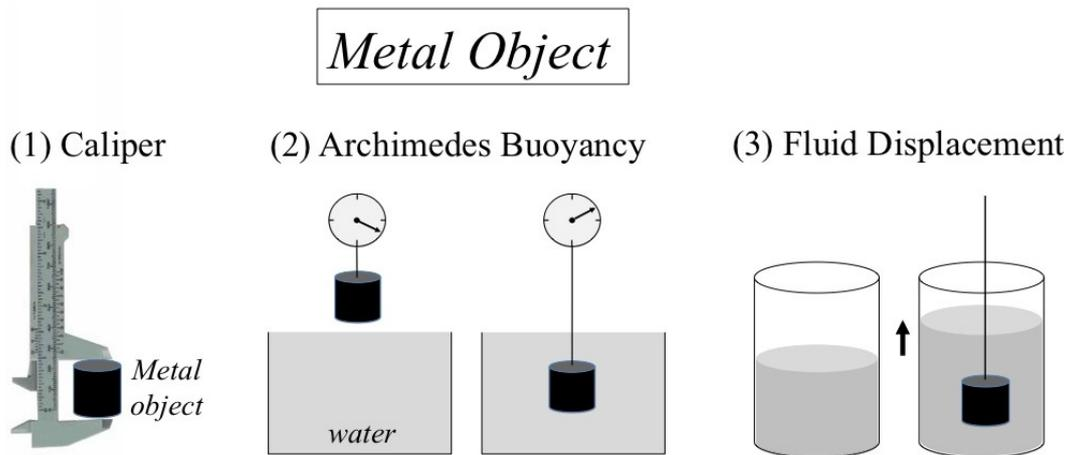
**Fig.2** Three ways of measuring a metal object's volume  $V$ .
