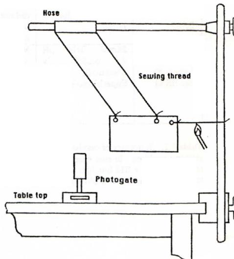
**Figure 1:** Pendulum at rest at height  $h_0$  with the photogate in position.
