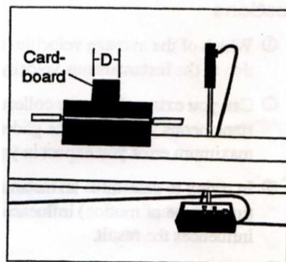
**Figure 2:** Measuring velocity in gate mode.
