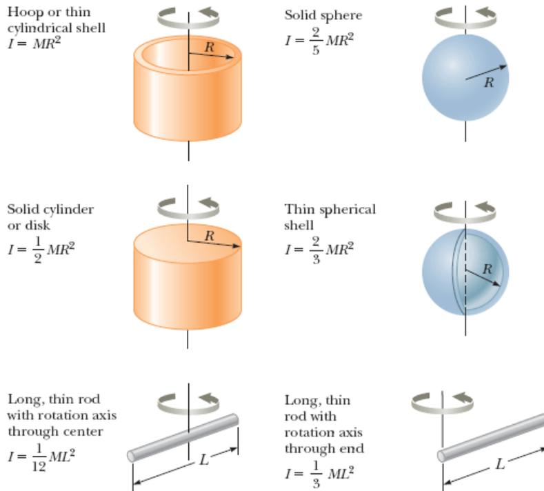
(a) Find the moment of inertia for each object as it rotates about the axes shown in the table above.
