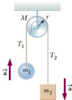
(a) Why must the tension  $T_2$  be greater than the tension  $T_1$ ?
